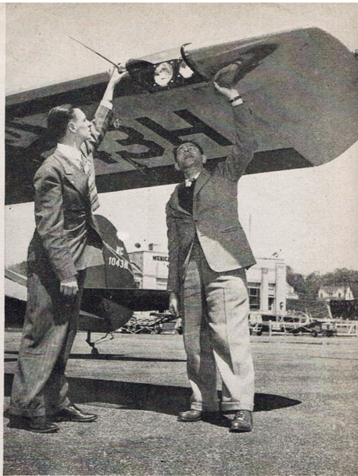
Arthur Dean, left, and Samuel Gordon, general observers, inspect landing lights on the new Aeronca. One points straight ahead, the other is canted downward for taxiing. Wing skin is all metal.
