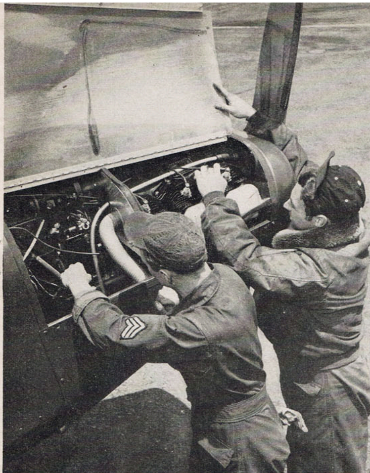
The team technicians, Bobby L. Diener and Francis J. LaPierre, check over the power plant installation. They reported that the engine and accessories were unusually accessible for servicing.
