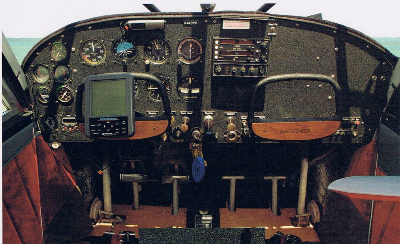
The panel is vintage 1940s, with the instruments clustered in the center for easy accessibility (above). Fuel management also takes place on the panel.
