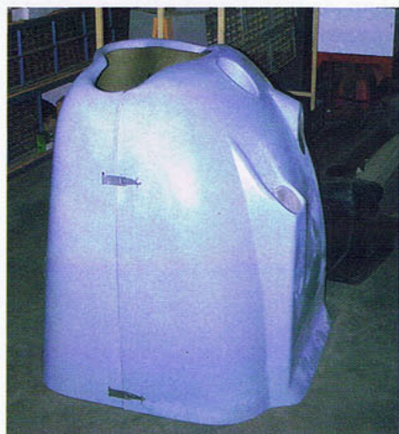
Burl Rogers displays several tooling dies used to manufacture Sedan elevators. Rogers's 180 hp conversion uses a modified Cherokee 180 cowl. Despite its size, the new cowl weighs only 26 lb.
