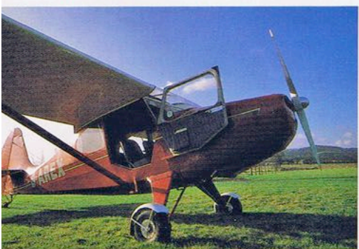
A long propeller for good low-speed thrust and wide splayed main gear legs for easy ground handling. Cabin area is generous and the wide doors make passenger-loading easy. (James Grimstead photos.)
