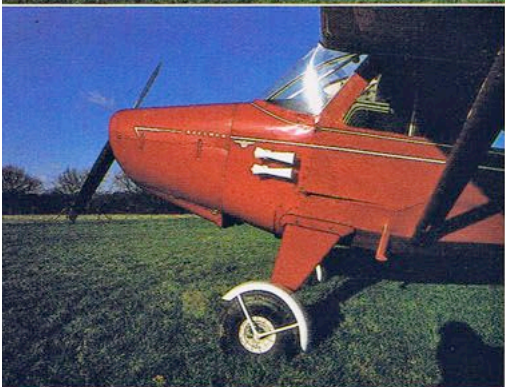
A long propeller for good low-speed thrust and wide splayed main gear legs for easy ground handling. Cabin area is generous and the wide doors make passenger-loading easy. (James Grimstead photos.)
