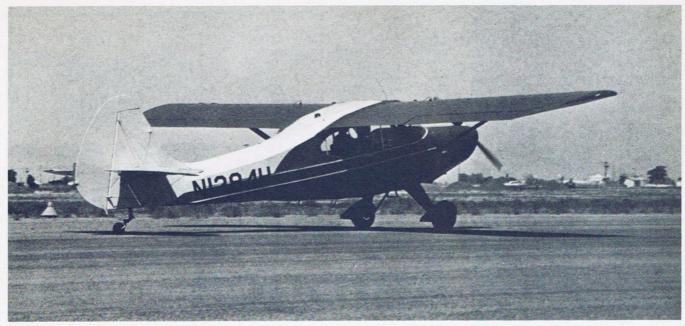
Fuselage pinches down aft of cabin, so headroom suffers in favor of lift and the sleek lines of a tapered fuselage.
