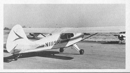
WALK-AROUND inspection of the ship reveals her lineage. The empennage especially hints strongly at the Aeronca line, and it is only the obviousness of the four seats that keeps a stranger from assuming that it is one. The gear and the shape of the windshield also point out that this is the big brother of the familiar Chiefs and Champs. The size of the rudder and vertical stabilizer attracts immediate attention and hints at the excellent ground handling characteristics.
