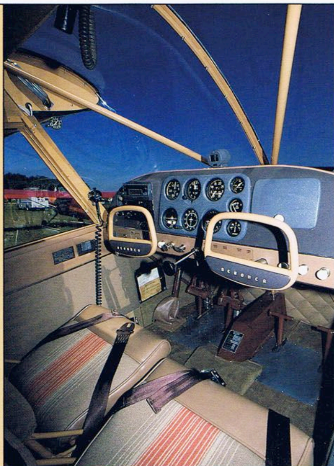
Carefully restored to almost original configuration, the cockpit of the Sedan shows off its spacious cabin width, and the great visibility out the large windshield. The only major difference between 1950's and now? The 6" radio stack on the left side of the panel.
