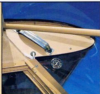
In keeping with the "keep it simple" school of thought, the fuel gauges for the wing-mounted tanks are graduated tubes.
