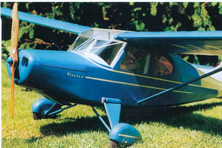
Sprung undercarriage pivots on a wire in a tube across the fuselage. Wheel spats are a prominent feature on N1491H.
