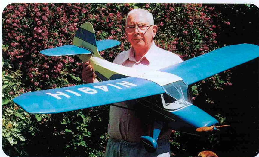
ABOVE: With its side-by-side seating, the 65" span Aeronca is quite a chunk of aeroplane. Ready to fly it weighs 48 ounces.
