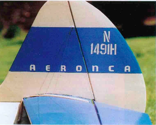
ABOVE LEFT: Finished effect of stencilled markings applied as described in the text. Tail unit is banded-on, as on the original Mercury kit plan which you can still get from Phil Smith. ABOVE RIGHT: Access to R/C gear through the non-scale roof hatches; if you finished the four-seat interior you could hide all the gear under the floor with access from below.
