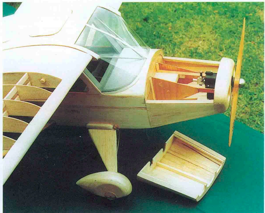
The original used an E.D. 2.46 sidwinder, but David has fitted a Rustler Lynx inverted, equipped with an R/C throttle.
