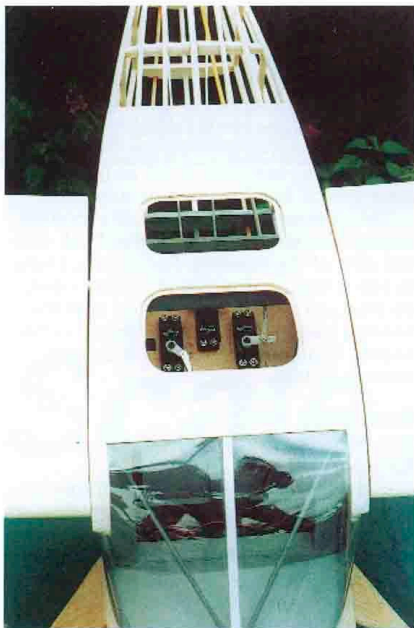
LEFT: Three standard servos look lost in the vast cabin. You could do a detailed interior and hide all the gear below the floor.
